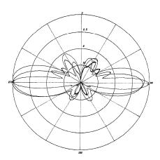
NCG SOMPANY Elevation pattern: This pattern represents the typical elevation pattern when the CX-333 is mounted in free space without interference from other metal objects. The inner most lobe is the 440MHz elevation pattern, the largest lobe is 146MHz elevation pattern. The lobe between is the 220MHz elevation pattern.
